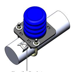
Mounting Bracket should be up against the wire harness bracket. Confirm that wiring is not streched or pinched.
