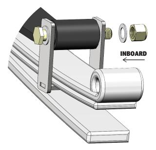
**11.** Using a heavy-duty C-Clamp or SuperSprings installation tool, compress the rear of the SuperSpring and attach the rear shackle in the same way as the front by repeating steps 9 and 10, without a Leaf Spring Isolator.
